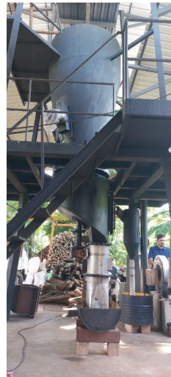
1(a) 1(b) Figure 4(a) & (b) – Design and fabrication of the charcoal generator
