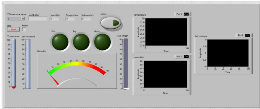
Figure 5: This figure displays the graphical user interface (GUI) of the automated plant watering system, developed using LabVIEW. The interface provides a comprehensive dashboard for monitoring and controlling the system.
