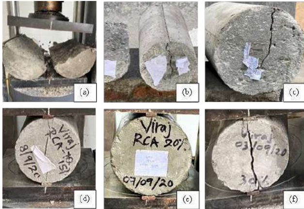
Figure 4. Cylinders after failure at 7 days
