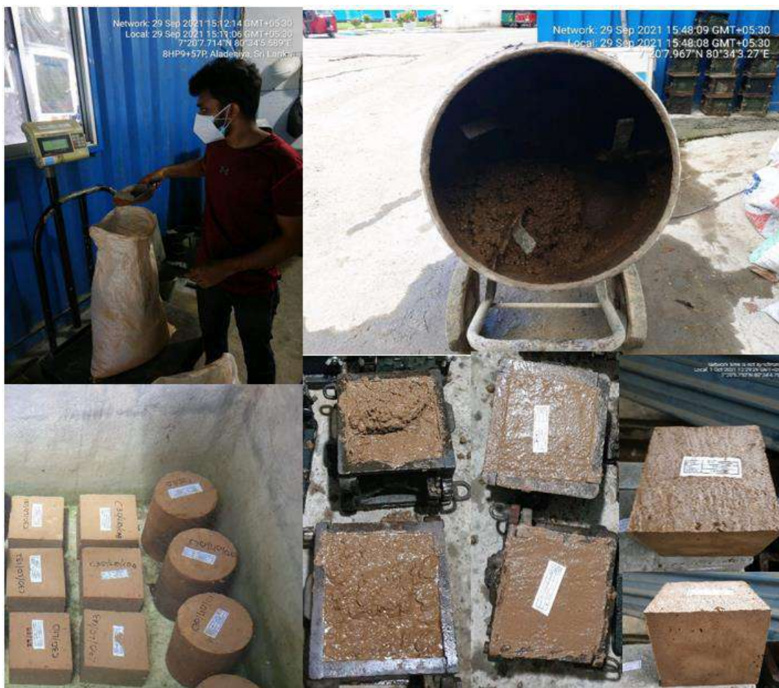
Figure 3.1 Concrete Casting and Curing
