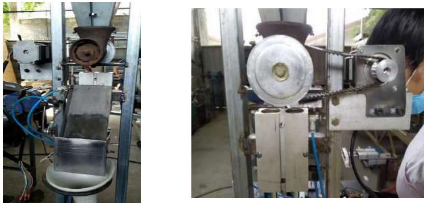
Figure 18. Mechanical structure of the filling section
