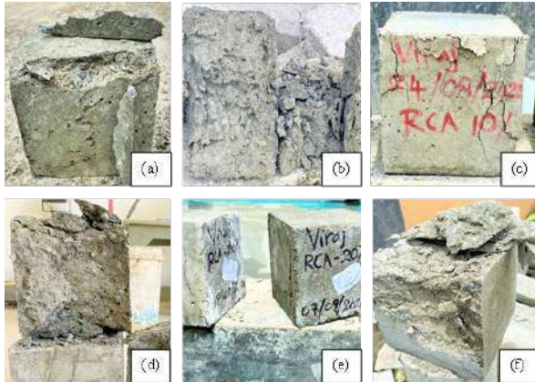
Figure 2. Cubes after failure in 7 days
