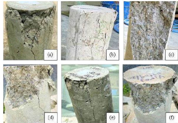
Figure 3. Cylinders after failure in 7 days
