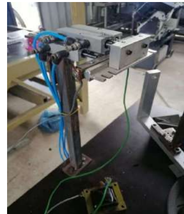
Figure 19. Mechanical structure of the sealing section
