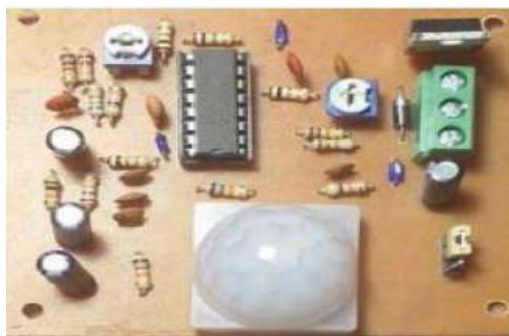
Figure 7. Constructed PIR sensor module
