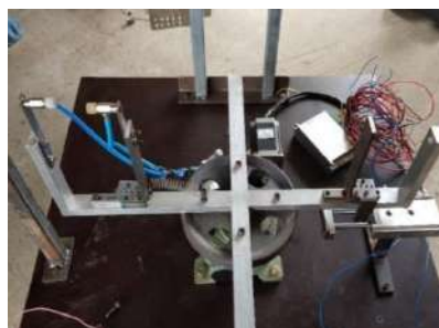
Figure 16. Mechanical structure of the packet moving system
