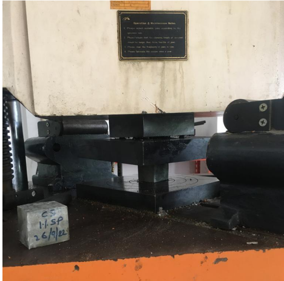
Figure 8: Compression test on a test specimen
